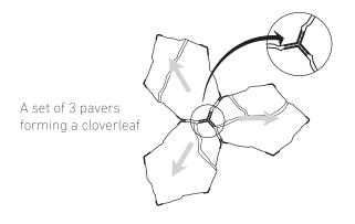
To make the installation easier, the front of the paver should point to the back of the other paver.
