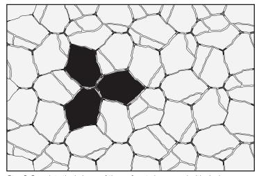
Step 3: Complete the balance of the surface to be covered with single pavers.
