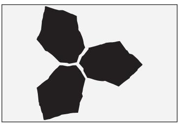
Step 1: Begin by laying 3 pavers at the center of the surface to be covered.
